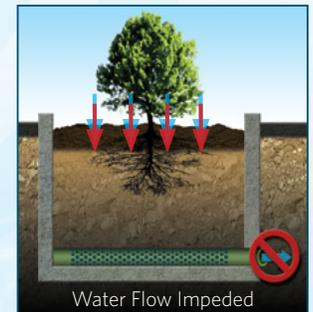
Sediments accumulate on top of the media leading to clogging.
