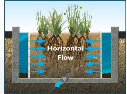
Sediments accumulate adjacent to vertical media surface reducing clogging.
