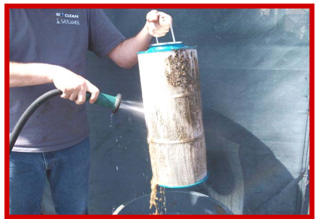
To Wash Cartridges Remove from Vault. Place Over Trash Can and Use a Garden Hose to Spray Clean.
